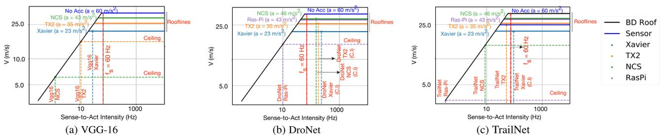
Fig. 4. The F-1 roofline plots for three end-to-end learning models running on Nvidia Xavier/TX2, Intel NCS, and Ras-Pi.  $C/I$  is the throughput of running a control algorithm on a given hardware, shown only when it is greater than  $f_s$  (sense-to-act intensity is equal to  $f_s$  in these cases).
